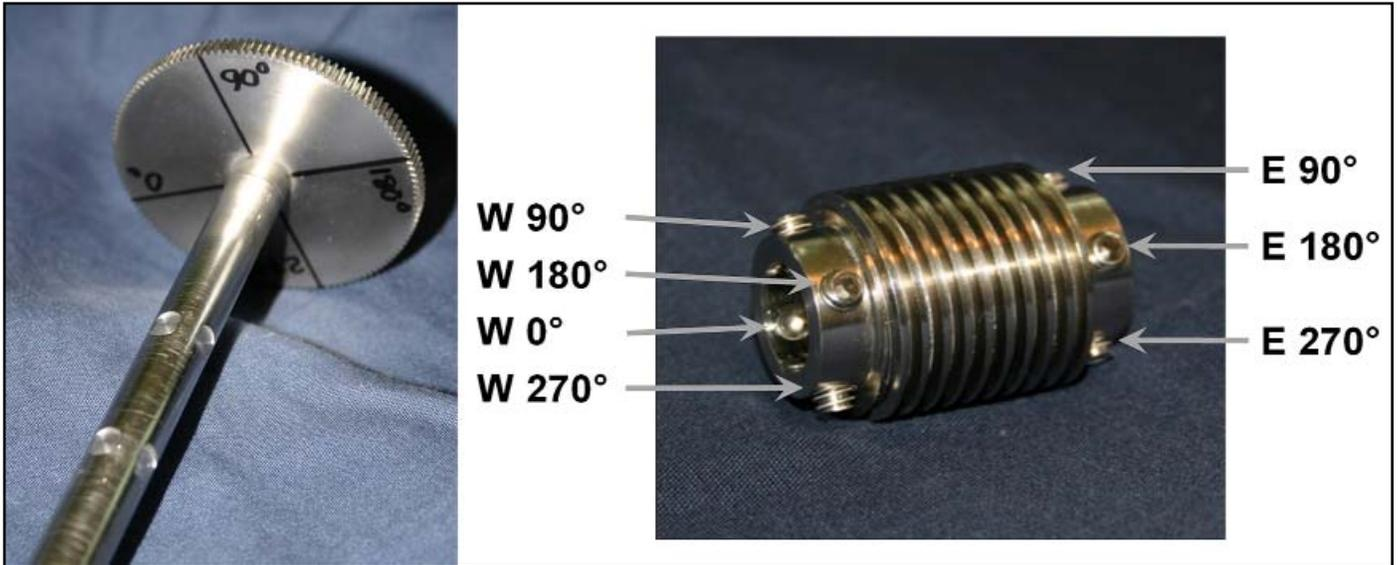
**Figure 2.** The mount's RA two-piece worm with orthogonal set screws that not only affix but also align the worm on its shaft (shown to the left). Each set screw has a unique identifier to enable appropriate corrections to the PE.
