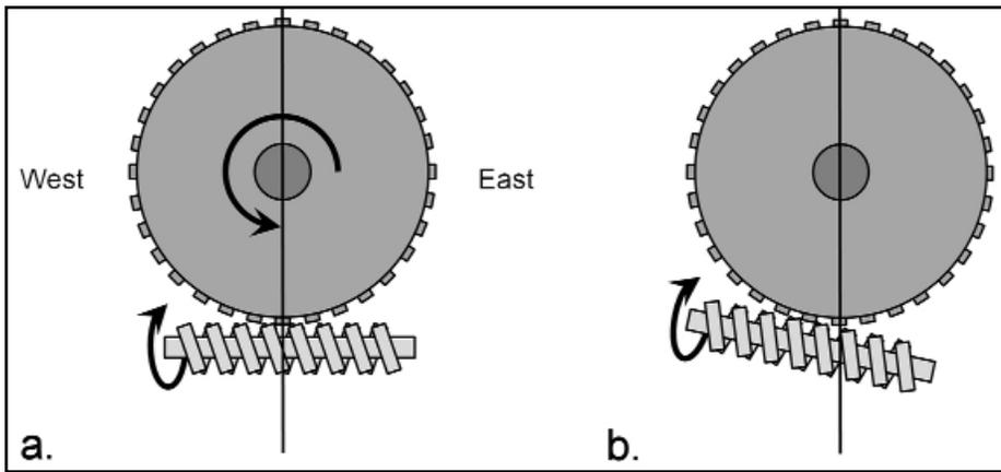
**Figure 3.** *Fundamental mechanical elements of a worm gear utilized in a telescope's RA drive. Panel a: A rotating worm gear held in a fixed position causes the clock gear to rotate and compensate for the Earth's rotation (the RA axis is aligned to the celestial pole, which in the northern hemisphere points north with an altitude equal to the latitude). Panel b: the rotating worm will travel around a stationary clock gear if the worm is not held in a fixed position relative to the gear.*
