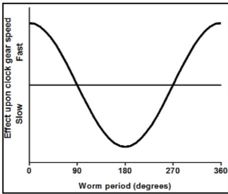
**Figure 5.** The effect of the worm misalignment in Figure 4 upon the clock gear speed. The horizontal line represents the nominal clock gear speed.
