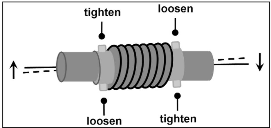
**Figure 6.** Set screws on a two-piece worm permit adjustment to align the worm on its shaft. In this figure the adjustments would correct for the misalignment corresponding to that shown in Fig. 2a.
